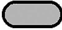
FIGURE 3.4 Cross section of enameled round wire after flattening. (By permission of ABB Inc., Jefferson City, MO.)
