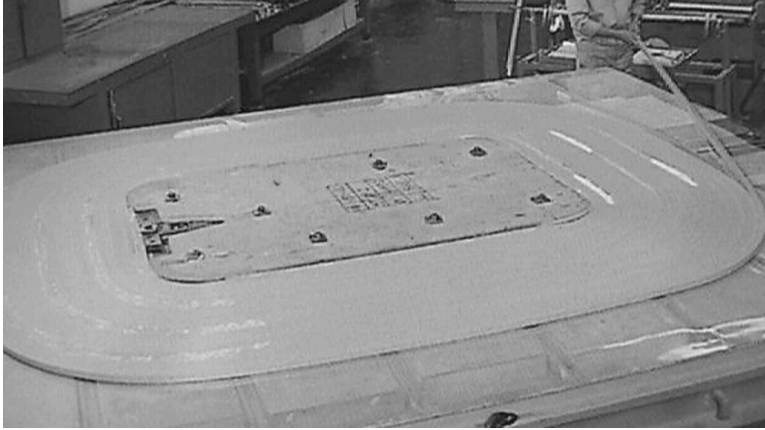
FIGURE 2.12 Pancake winding during winding process.
